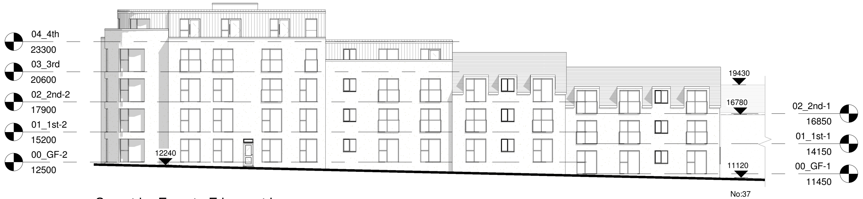
South East Elevation 1 : 200
